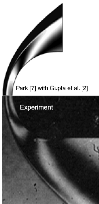
Fig. 18 Fringe patterns on 1-in.-diam cylinder with Park [7] model and Gupta et al. [2] equilibrium constant.
